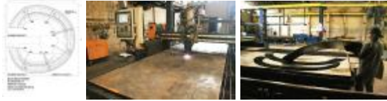
Figure 10. CNC plasma cutting process (images by Wilson Barbosa).
