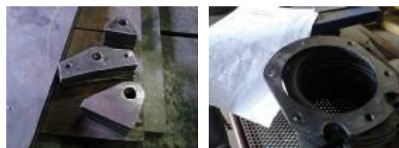
Figure 1. Parts commonly produced by the company's CNC plasma cut machines (photo by Wilson Barbosa).
